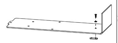
Do not fully tighten the screw and the nut, leave them loose for inserting into T-slot.
