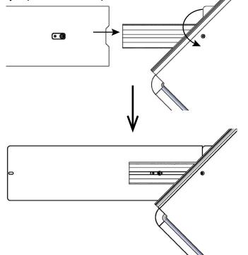
Step 5. Rotate the Snap Frame back to its display position and align the top hole with the top slot on the Acrylic. Screw (1) M4X14mm throught the aligned holes from the front and tighten it with (1) Square Nut.
