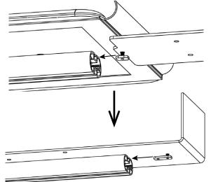
Step 4. Assemble (1) M4X10mm screw, (1) M4 washer and (1) Rectangle T-slot nut at the lower hole of the Top Acrylic. Remove the end cap from the top of the pole. Pivot the snap frame to the side.
