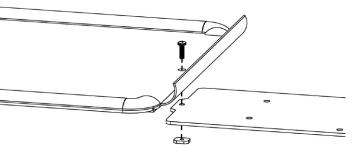
Do not fully tighten the screw and the nut. Leave a gap between nuts and the Bent Acrylic
